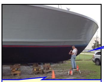
(Above) Al works on painting the water line mark on the PTF-3.
